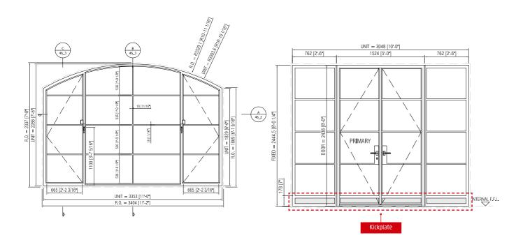
A classic design feature is the small insulated kick- at the base to both shield the glass from any impact, but combinations. Considering the small profile of about during rainy spells. Brombal's steel doors, the architect wanted a little extra
